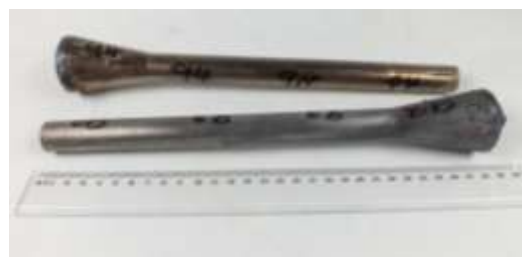
Fig. 2 Alloys after VIM a centrifugal casting.
