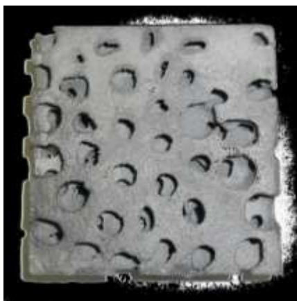
Fig. 6 Casting (cast iron with lamellar graphite) – type A
