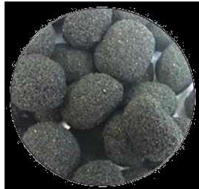
Fig. 9 Precursors – Furan molding mixture (regular shape and size)
