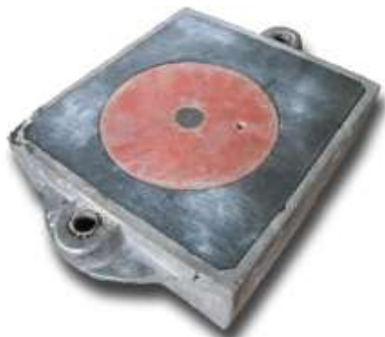
Fig. 2 Mold made from commonly used green sand
