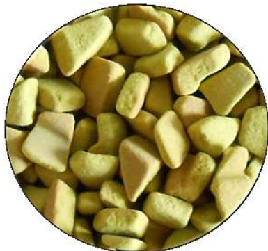
Fig. 8 Precursors – Croning process (irregular shape and size)
