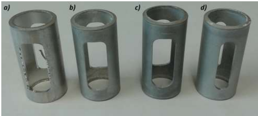
Fig. 4 Machining parts: a) before finishing, b) after time of machining 60 min, 3000 Hz, 15 % abrasion degree, c) after 60 min, 3000 Hz, 85 % abrasion degree d) after 60 min, 3000 Hz, 85 % abrasion degree.
