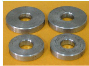
Fig.3. Couples of rollers corresponding to different sliding degrees \xi [6,8]
