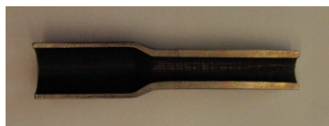
Fig. 4 Examples of experimentally rolled MT1020 steel reducing tubes at s_0/D=0.09 and K=1.46 ratios, where: a) reducing tube, b) longitudinal section of the reducing tube
