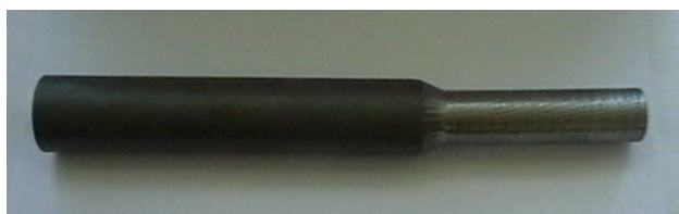
Fig. 4 Examples of experimentally rolled MT1020 steel reducing tubes at s_0/D=0.09 and K=1.46 ratios, where: a) reducing tube, b) longitudinal section of the reducing tube
