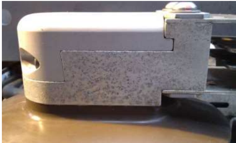
Fig. 2 Failure of silver coating on aluminium
