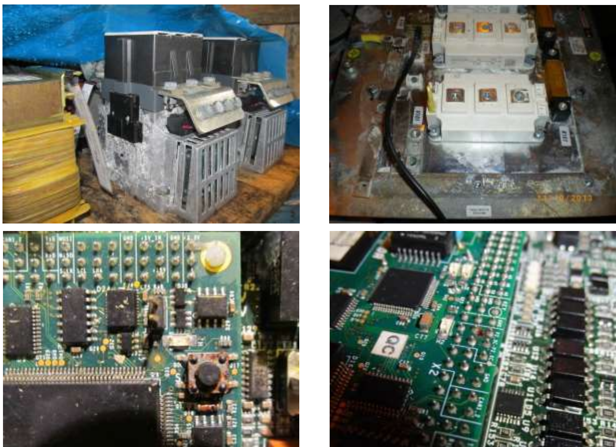
Fig. 4 Electric and electronic elements' corrosion caused by non-suitable protection during transport
