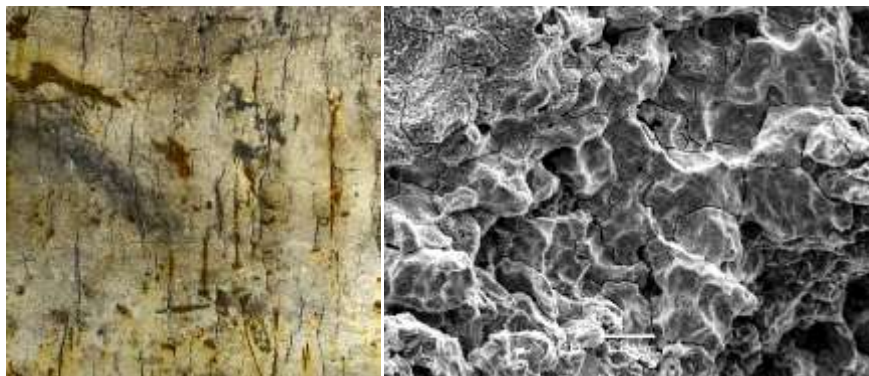
Fig. 4 Network of cracks on the outer pipe surface and fracture surface morphology
