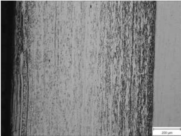
a) microstructure of X7CrNiNb18-10 steel - longitudinal section
