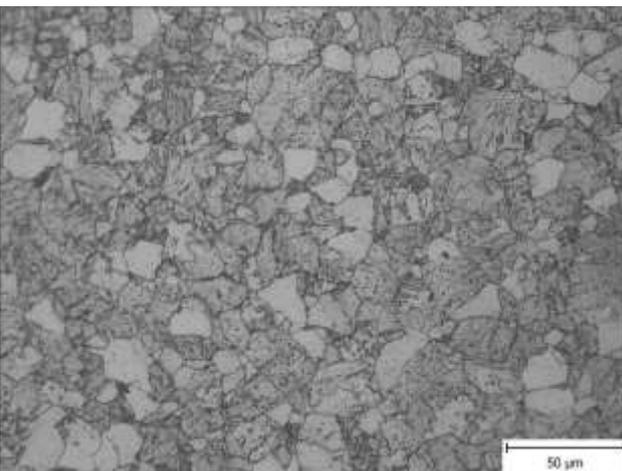
e) microstructure of 11CrNi9-10 steel longitudinal section – mid-thickness of the shell
