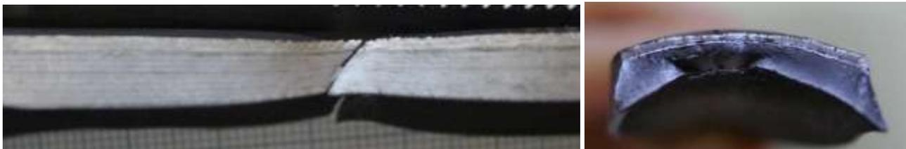
a) sample after tensile test at room temperature
