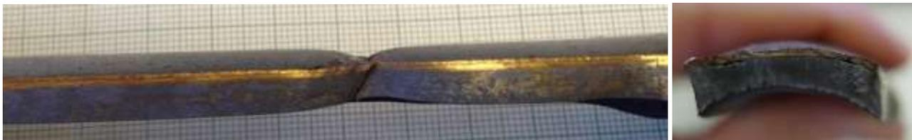
b) sample after tensile test at elevated temperature (450°C)
