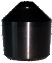
Fig. 1 Photograph of a sample used in the tribological tests.
