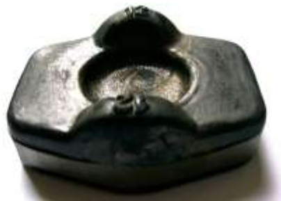
Fig. 8 P/M FeAl alloy part forged at 900°C
