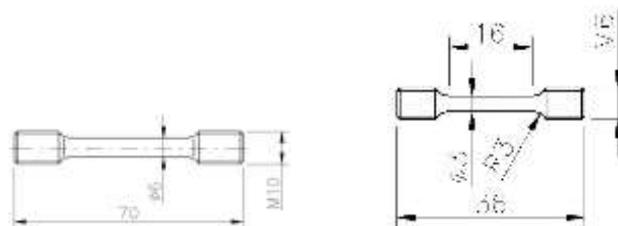
**Fig. 2** Tensile test specimens
