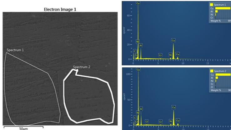
**Fig. 2** EDS Spectrum of Sample 1.
