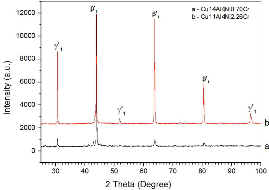
**Fig. 3** XDR result of Sample 1 (a) and Sample 3 (b).
