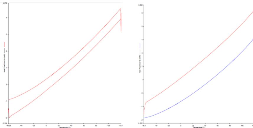
**Fig. 5** DSC result of Samples 2, to the left, and 3, to the right.
