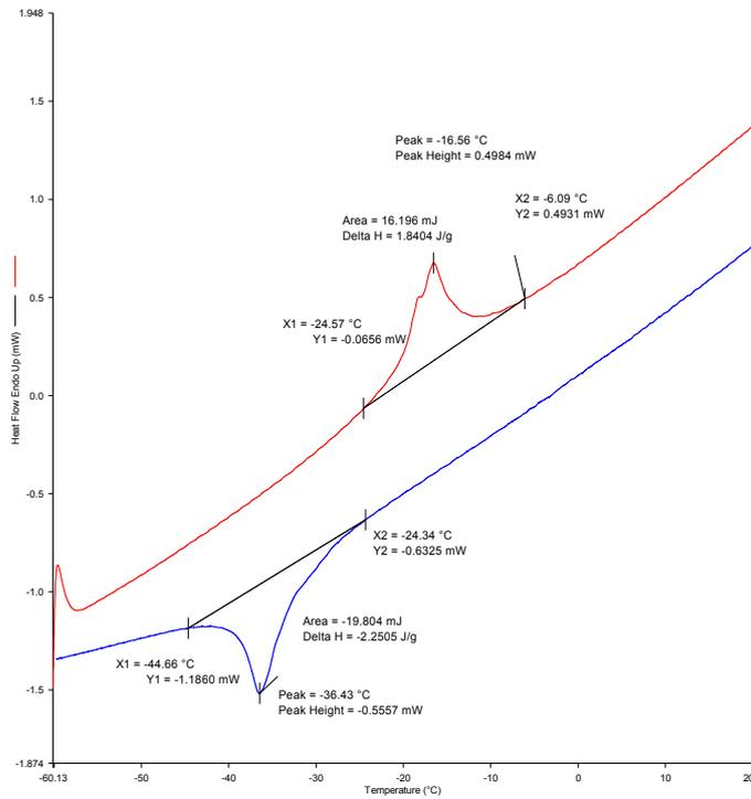
**Fig. 4** – DSC result of Sample 1, 0.74% of Chromium in CuAlNi alloy.
