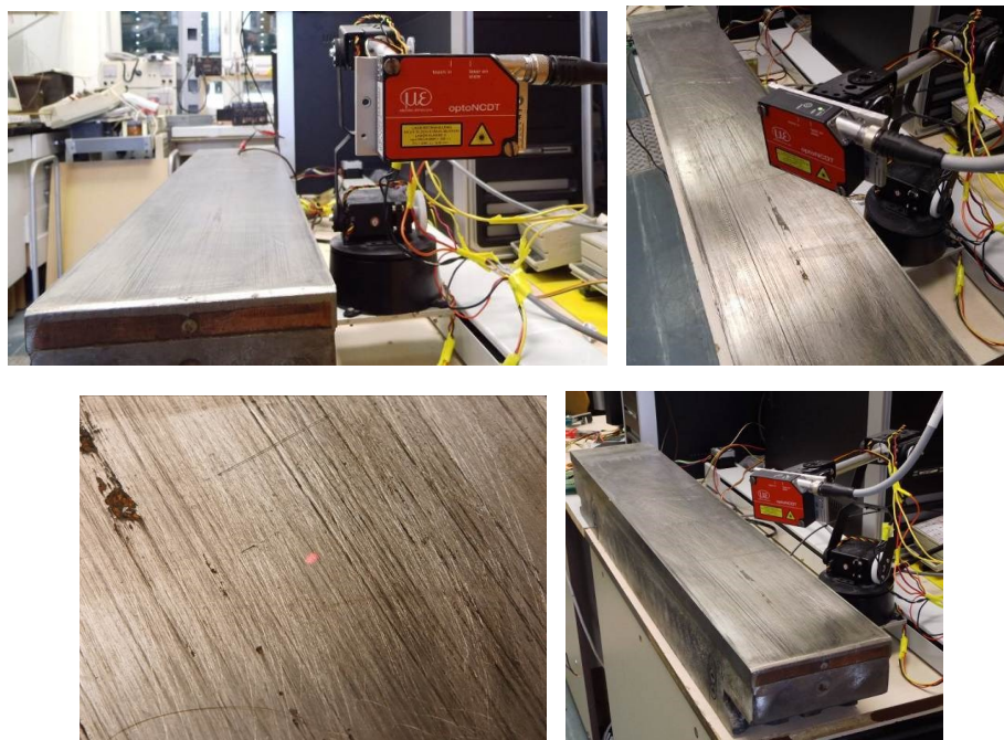
Fig. 4 View of the measuring assembly for verification of the surface - the wear surface metallurgical materials (measurements in laboratory conditions VSB - Technical University of Ostrava)
