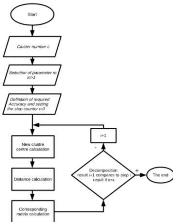
Fig. 1 Algorithm of method of fuzzy k-Means
