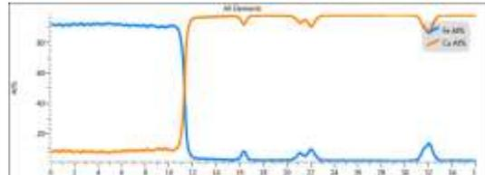
**Fig. 19:** Linescan analyze made on sample annealed at 1100 °C
