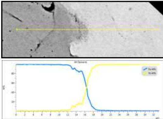
**Fig. 25:** Linescan analysis made on the sample annealed at 500 °C
