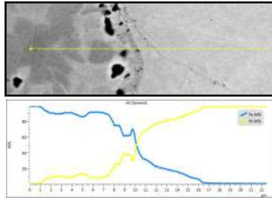
**Fig. 26:** Linescan analysis made on the sample annealed at 700 °C
