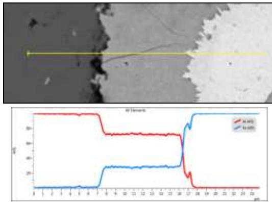
**Fig. 6** Linescan analysis, red line – aluminium, blue line – iron
