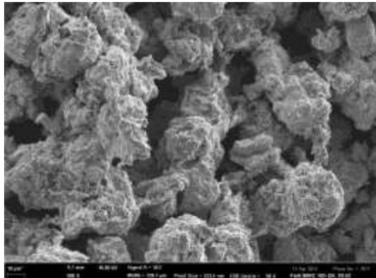
**Fig. 12:** Fracture surface of sample annealed at 600 °C
