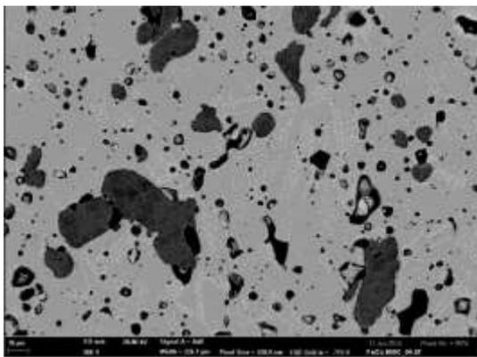
**Fig. 16:** Microstructure of sample annealed at 900 °C
