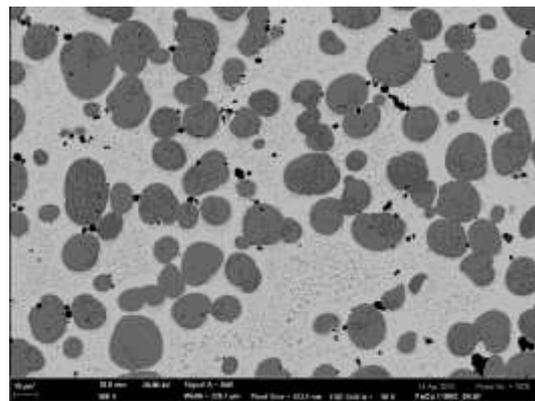
**Fig. 17:** Microstructure of sample annealed at 1100 °C
