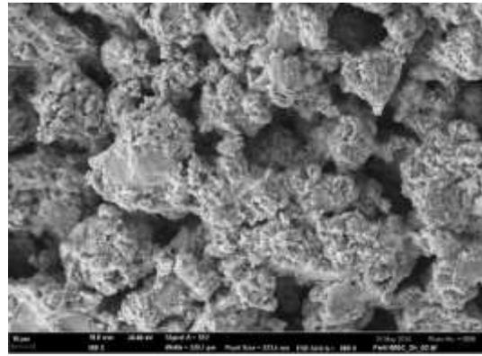
**Fig. 13:** Fracture surface of sample annealed at 650 °C
