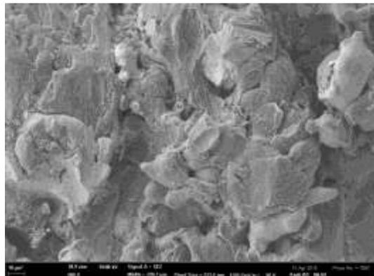
**Fig. 4** Fracture of the as deposited material
