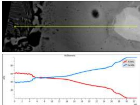
**Fig. 11** Linescan analyze made on sample annealed at 650 °C
