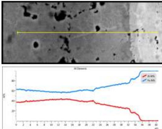
**Fig. 10** Linescan analyze made on sample annealed at 600 °C
