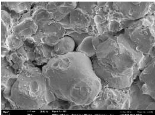
**Fig. 27:** Fracture of annealed material at 500 °C
