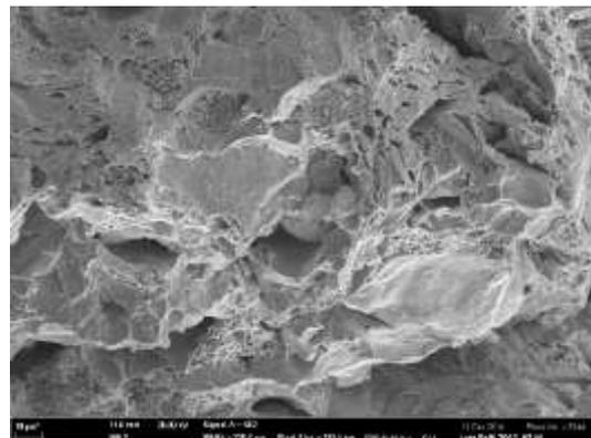
**Fig. 28:** Fracture of annealed material at 700 °C
