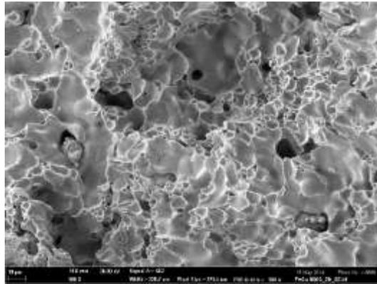
**Fig 20:** Fracture of sample annealed at 900 °C
