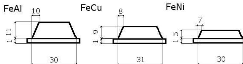
**Fig. 2** Scheme of mechanical dimensions of the deposits
