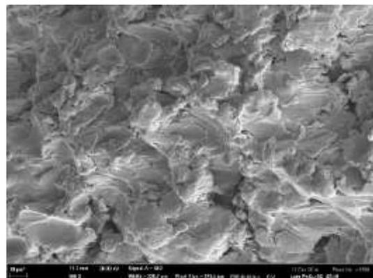
**Fig. 15:** Fracture of the as deposit material
