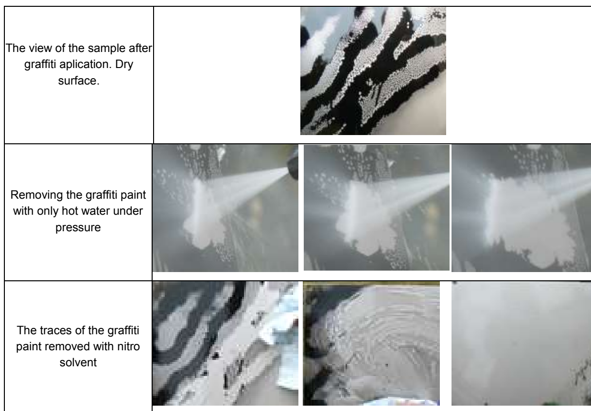
Fig. 1 Steps in removing spray paint from anti-graffiti coatings
