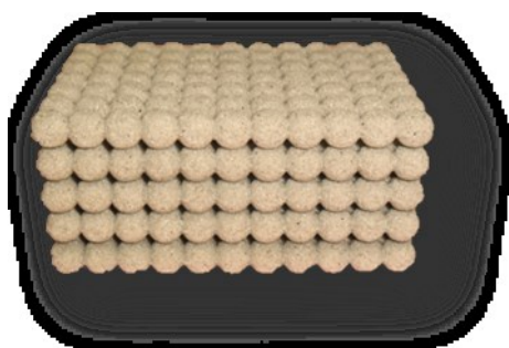
Fig. 3 Core (preform) composed of five layers of cells
