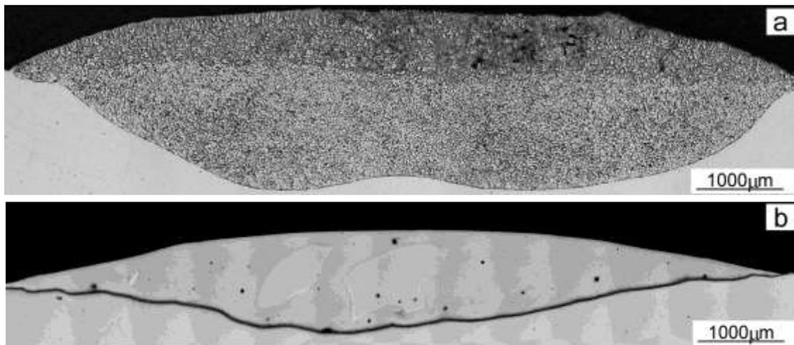
**Fig. 1.** Cross-sections of magnesium samples surface-alloyed with aluminium using the TIG method: (a) at a higher current (40 A), (b) at a lower current (25 A).
