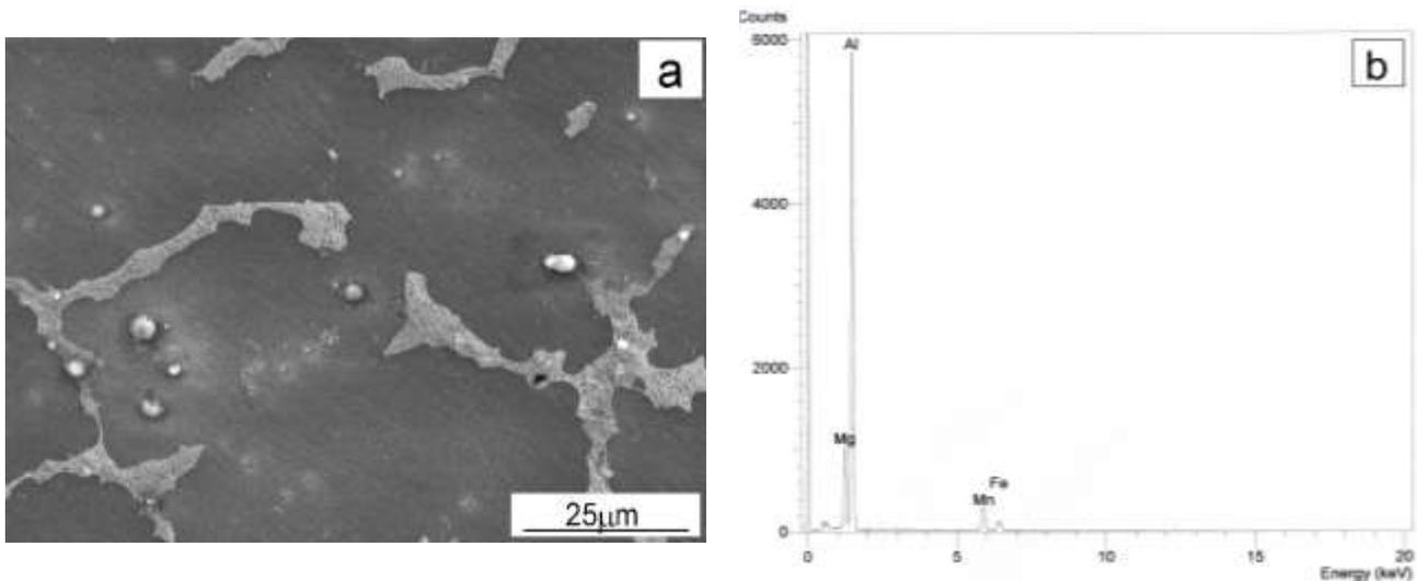
**Fig. 4.** (a) Distribution of white particles in the alloyed layer, (b) X-ray spectrum for a white particle.
