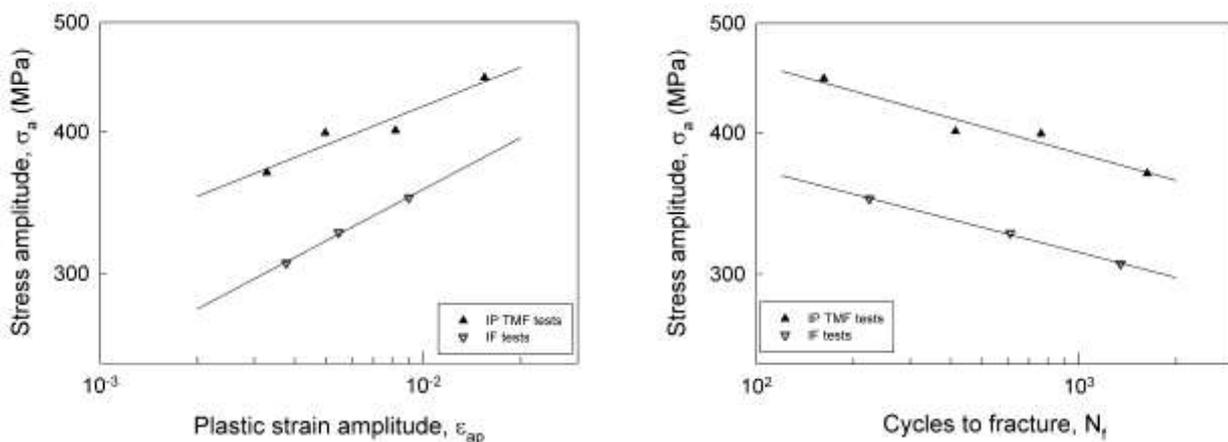
**Fig. 3.** Fatigue life curves for IP TMF and IF cycling (a) CSSCs and (b) Wöhler-Basquin
