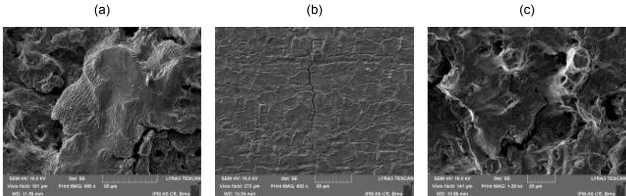
**Fig. 4.** (a) Transgranular cracking with striations under IF cycling, (b) and (c) mixed mode cracking under IP TMF cycling.
