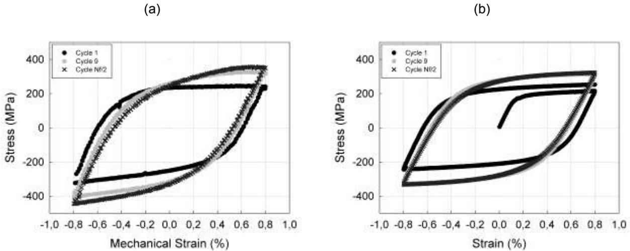
**Fig. 1.** Stress-strain hysteresis loops at  $N = 2, 9$  and  $N_f / 2$  of AISI 316L (a) IP TMF cycling at  $\Delta\epsilon_{mech} / 2 = 8 \times 10^{-3}$  and (b) IF cycling at  $\Delta\epsilon / 2 = 8 \times 10^{-3}$
