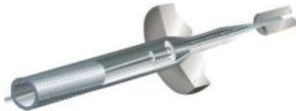
Fig. 1 Tube drawing example using plug drawing technology [3]
