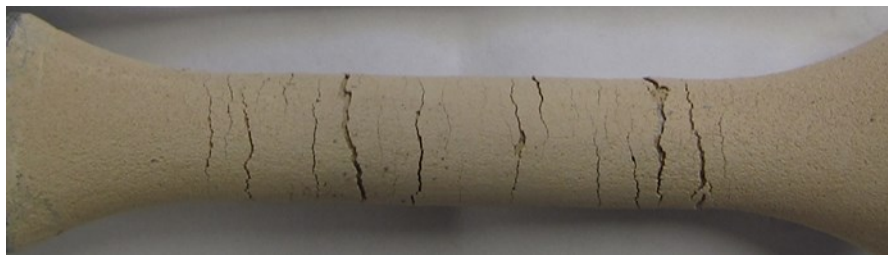
Fig. 3: The sample with the ZYP Coating CeO 2 after a cyclic loading test.
