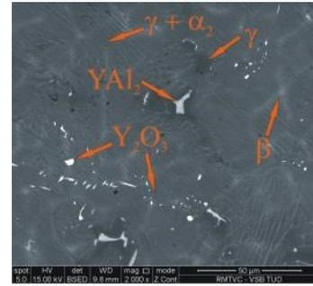
**Fig. 4** BSE image of 8Nb-Y-plasma sample
