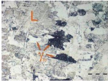
**Fig. 5** Microstructure of the 8Nb-plasma sample after the dissolving annealing (OM)
