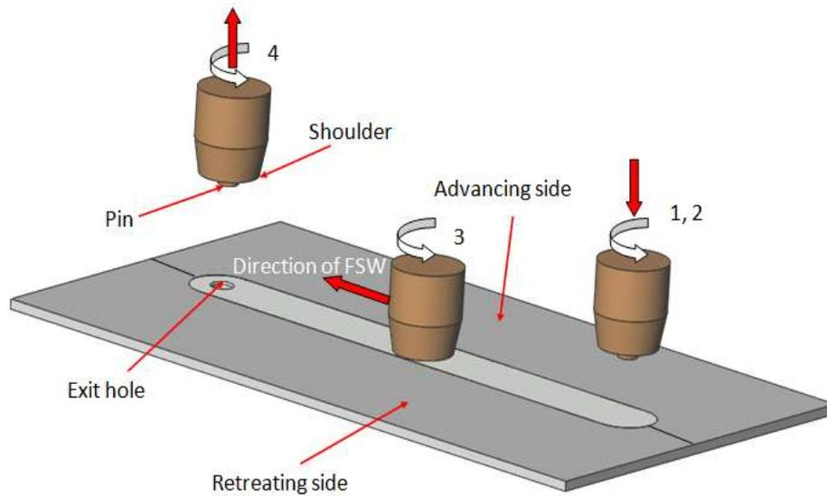
**Fig.1** Principal scheme of FSW
