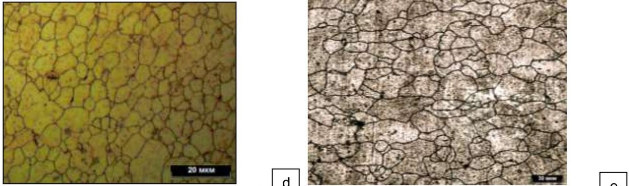
**Fig. 7** FSW samples: a) Macrosample of FSW nugget with 710 rpm, WS of 400 mm/sec; b) Microstructure of FSW nugget (710 rpm); c) Microstructure of FSW nugget (900 rpm); d) Microstructure of FSW nugget (1120 rpm); e) Parent metal.
