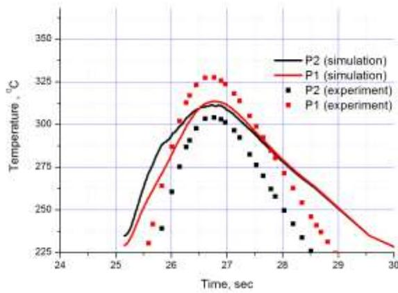
**Fig.6** Measured and calculated temperature during FSW (710 rpm, 400 mm/min of WS).
