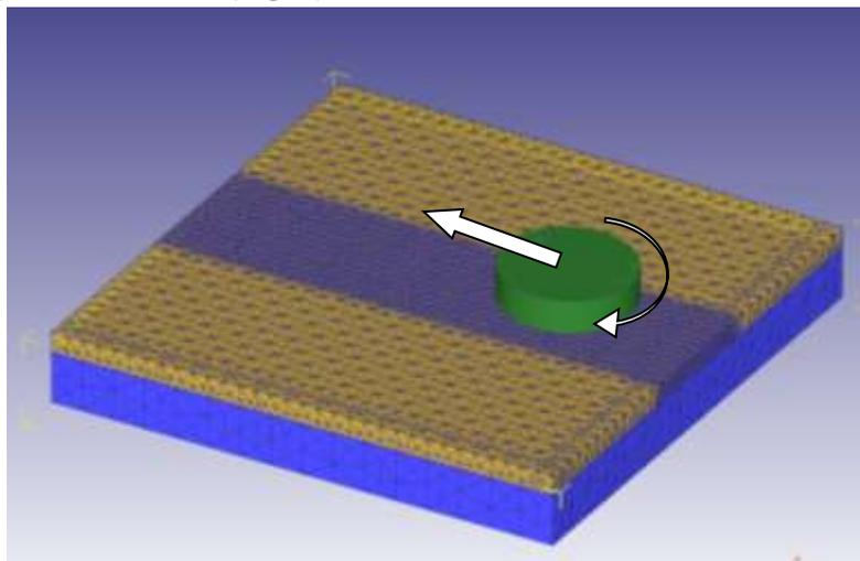
**Fig.2** FSW simulation model
