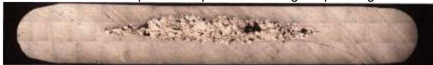
Fig. 8. The macrostructure of the sample after hot rolling without equal channel angular pressing
