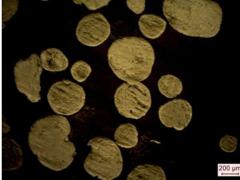
Fig. 1 Shape of powder particles Al + 15% (wt.) After the mechanical alloying REE
