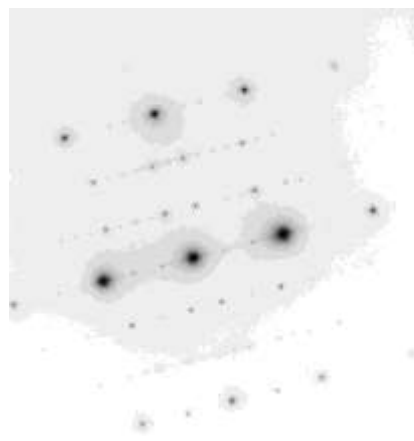
Fig. 10 Overlapping of [1-100]_{\alpha\text{-Mg}} and [1-100]_{\beta} zones in ED of the WEZM3211 alloy annealed up to 330 °C
