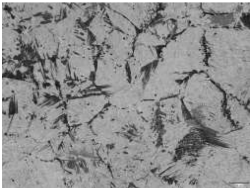
Fig.3. Weld metal microstructure sample no.9, Nital etched.
