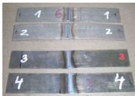
Fig. 1. Welded samples. (1,2-after 6xDRECE,3,4-IS)
