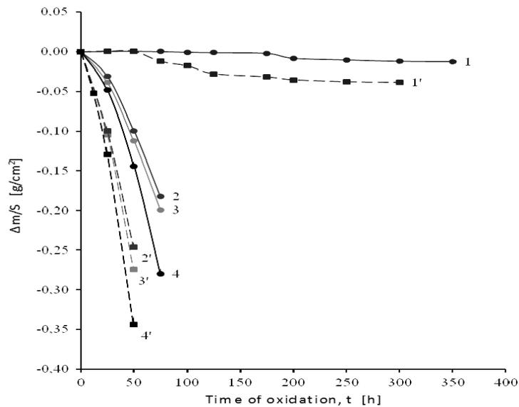
**Fig. 3** The comparison of oxidation rate of austenitic valve steels: 1 and 1' - X33CrNiMnN23-8, 2 and 2' - X50CrMnNiNbN21-9, 3 and 3' - X53CrMnNiN20-8, 4 and 4' - X55CrMnNiN20-8 in combustion gases from fuel oil with 5% and 10% additive of FAME [v/v]. Time of oxidation of tested steels is given in Table 2
