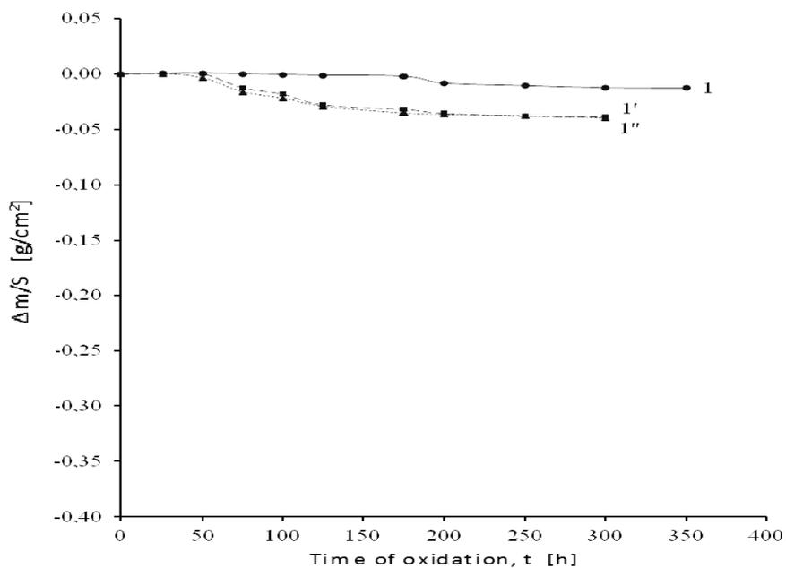
**Fig.4** The rate of oxidation of X33CrNiMnN23-8 austenitic valve steel in combustion gases from fuel oil with 5, 10 and 20% additive of FAME [v/v]. Time of oxidation of tested steels is given in Table 3
