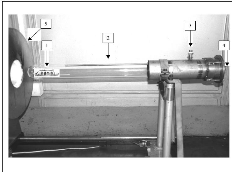
Fig. 2 Reactor used in corrosion resistance tests of valve steels in hot flux of exhaust gases from a combustion engine: 1 – samples in the glass tube of the reactor, 2 steel pipe used to deliver exhaust gases, 3 connector pipe delivering the combustion gases to reactor, 4 – combustion outlet, 5 – furnace used to increase the temperature of the combustion
