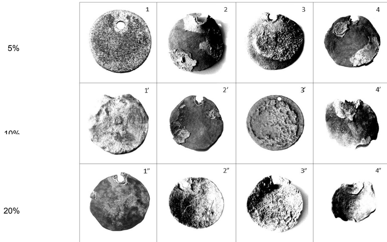
Fig.5 The macrographs of austenitic valve steels: 1 - X33CrNiMnN23-8, 2 - X50CrMnNiNbN21-9, 3 - X53CrMnNiN20-8 and 4 - X55CrMnNiN20-8 in combustion gases from fuel oil with 5, 10, 20% additive of FAME [v/v]. Time of oxidation of tested steels is given in Table 2 - 4 and in Figs. 3 - 5
