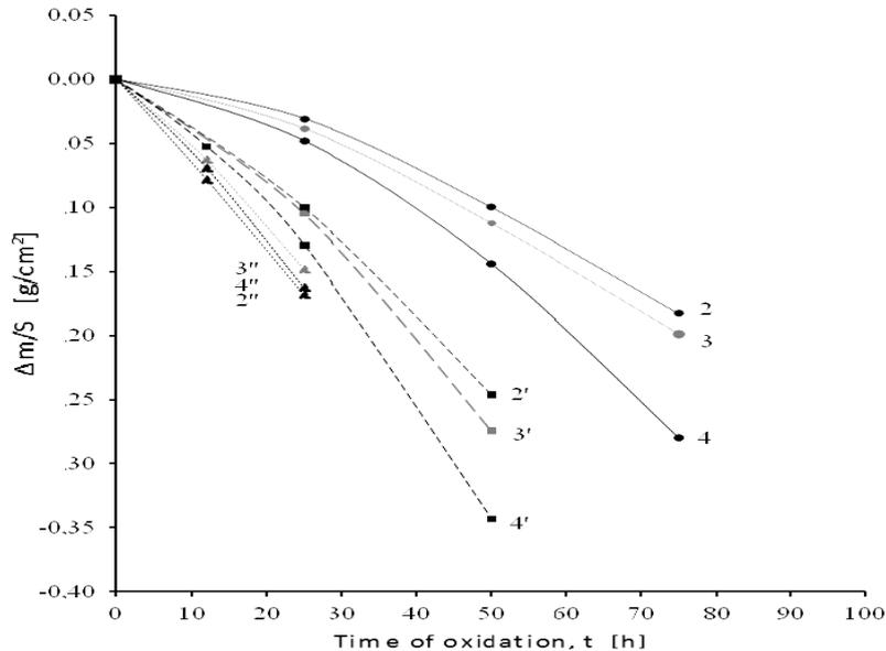
Fig.5 The comparison of oxidation rate of austenitic valve steels: 2, 2' and 2'' - X50CrMnNiNbN21-9, 3, 3' and 3''- X53CrMnNiN20-8, 4, 4', 4'' - X55CrMnNiN20-8 in combustion gases from fuel oil with 5, 10, 20% additive of FAME [v/v]. Time of oxidation of tested steels is given in Table 4
