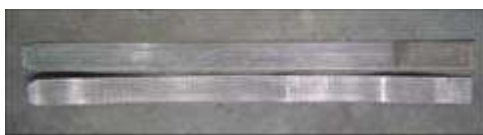
Fig. 3 Specimens of strip sheet AlMn1Cu alloy after the 8 th pass through DRECE machine
