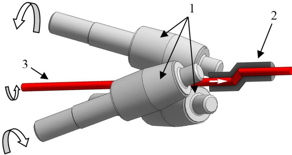
1 – conic rolls; 2 – stepped ECAP matrix; 3 – bar
