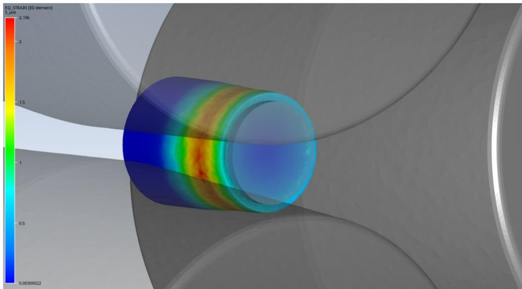
**Fig. 6** Strain on the billet during rolling
