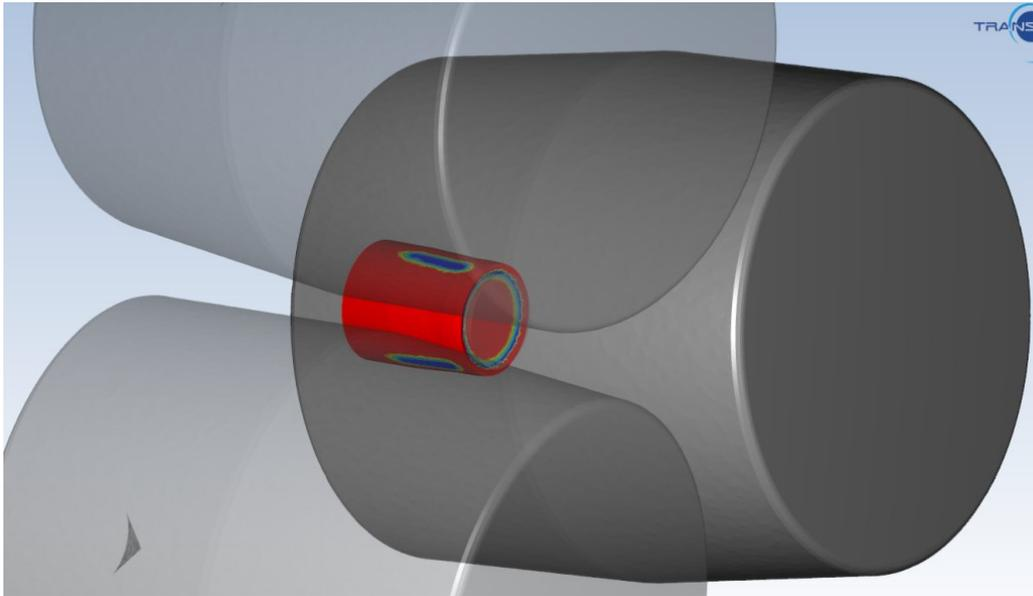
**Fig. 5** Contact area between the cylinder and billet
