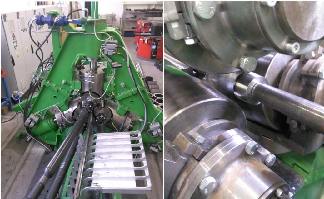
Fig. 2 Laboratory cross-rolling mill (MMR)
