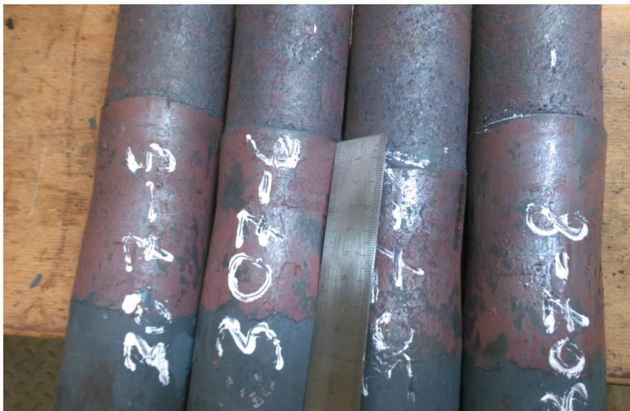
**Fig. 4** Rolling with visible deformation zone ( $\epsilon=10\%$ ;  $D_v/D_0=4,3$ )
