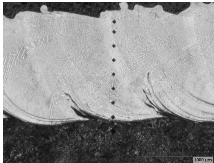
Fig. 5 Hardness measurement on cross section of cladded stellite coating.
