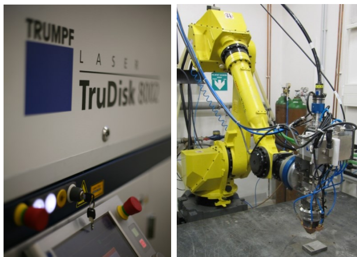
Fig. 1 The cladding system.
