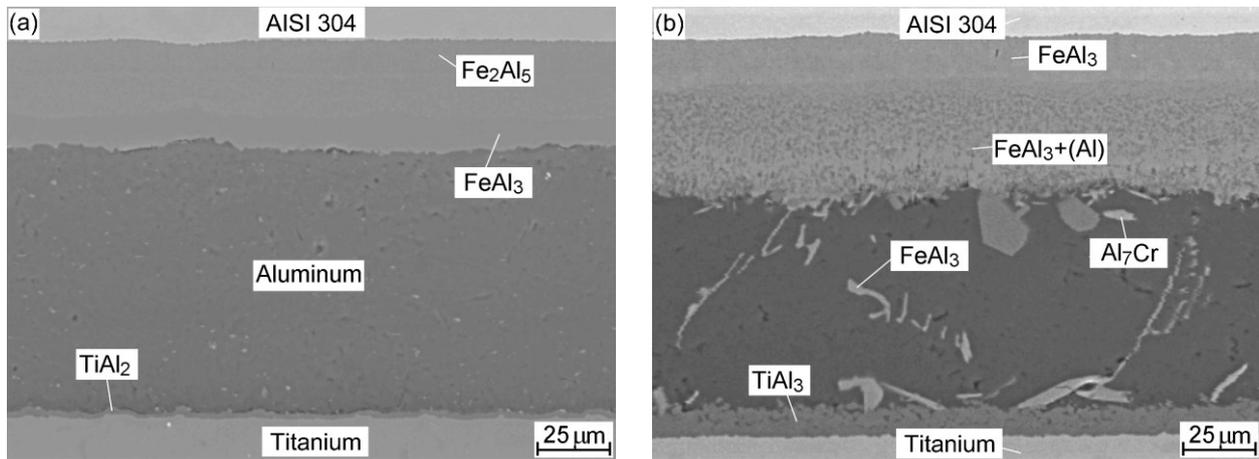
**Fig. 2** SEM images of the bonded joints processed at 650 °C (a) and 700 °C (b)
