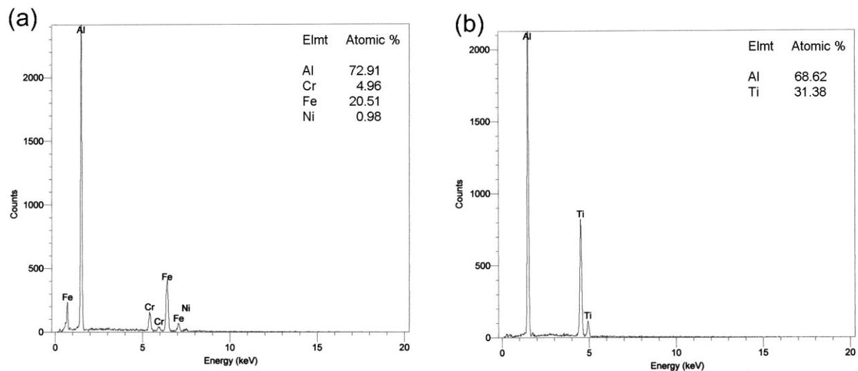
**Fig. 3** X-ray spectrums for  $Fe_2Al_5$  (a) and  $TiAl_2$  (b) intermetallic phases
