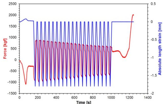
**Fig. 2** Evolution of force and strain in dependence on time at the test with 10-cycle strain (sample D6)
