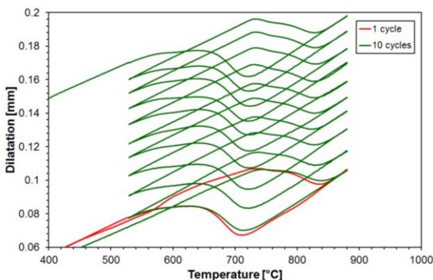
**Fig. 1** Example of dilatation of samples during tests with cycling change of temperature
