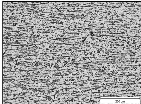
**Fig. 5** Microstructure of the sample after continuous compression test at the temperature of 880  $^{\circ}\text{C}$
