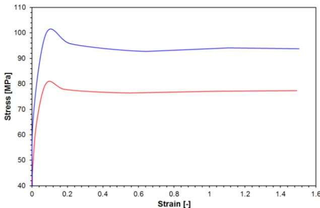
**Fig. 4** Stress-strain curves obtained by continuous tests by uniaxial compression
