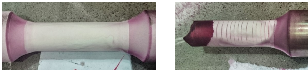
Fig. 3 Capillary testing of \text{Cr}_3\text{C}_2\text{-NiCr} coating at 20 °C (Left – sample with load under the fatigue life limit, right – sample above fatigue life limit)
