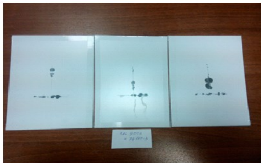
Fig. 3 The images of the samples №1 (a), № 2 (b) and №3 (c) after the experiment on saline mist.
