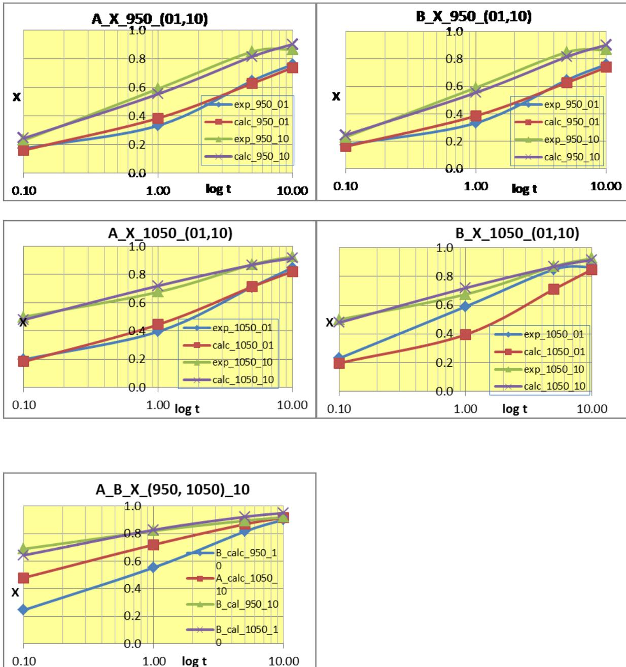
**Fig. 5** Avrami curves for various samples (A\_1183 (12 % Mn) B\_1184 (22 % Mn) and temperatures and strain rates.
