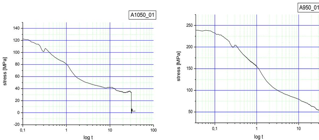
**Fig. 4** Stress-relaxation curves for **A\_1183** (13% Mn at temperature 1050 °C and strain rate 0,1 s<sup>-1</sup>) – left and for **A\_1183** (13% Mn at temperature 950 °C and strain rate 0,1 s<sup>-1</sup>) - right
