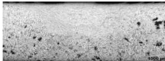
**Fig. 4.** Typical cross-section of the processed surface area; light microscope, ( $\omega=560$  rpm,  $v=560$  mm/min)
