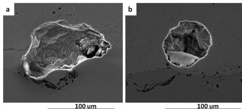
**Fig. 4** SEM of cavity formed on the coating/substrate boundary with contamination
