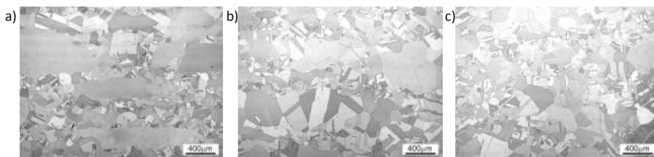
Fig. 2 The microstructure after supersaturation from temperature 1150 °C for the annealing time: a) 1 h, b) 2 h, c) 4 h
