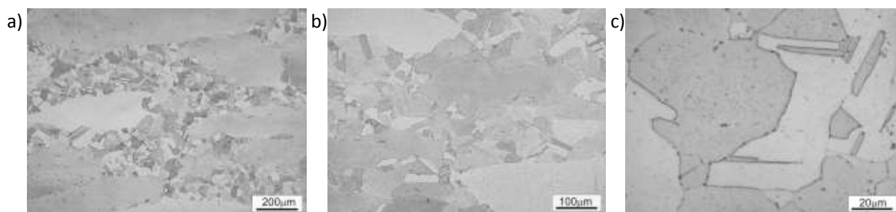
Fig. 1 Microstructure of the monel K-500 alloy, as delivered conditions
