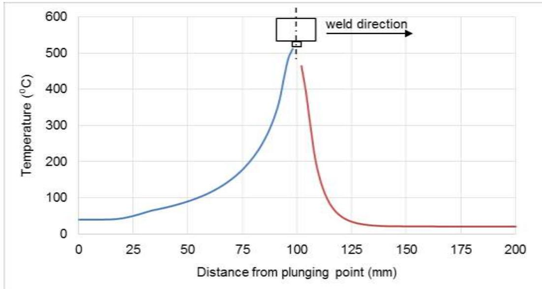
**Fig. 5.** Maximum temperature distribution along the weld centreline
