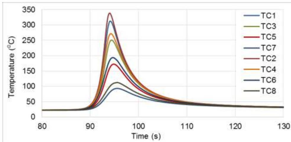
**Fig. 2.** Temperature cycles during FSW at 710 rpm
