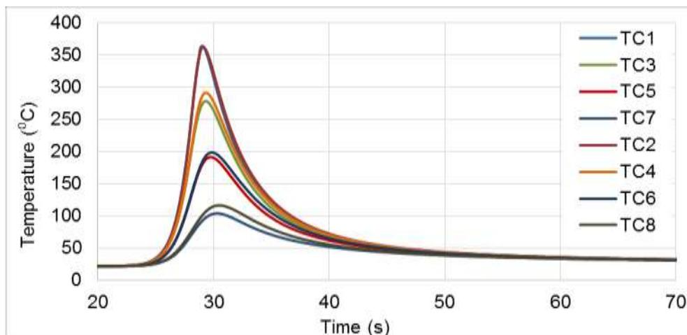
**Fig. 3.** Temperature cycles during FSW at 1120 rpm
