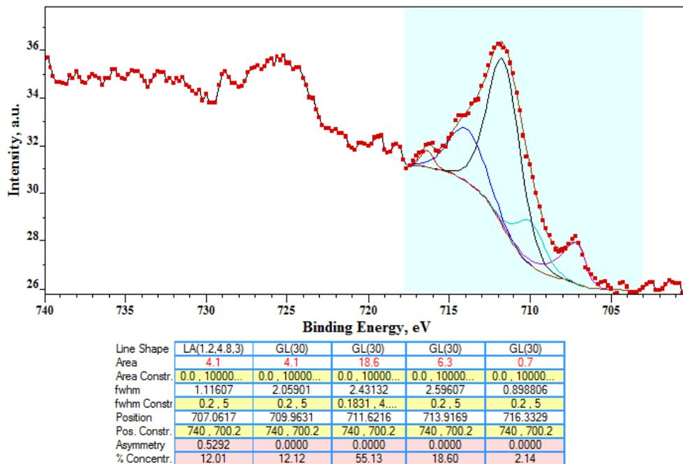
**Fig. 3** Fitting of Fe 2p<sub>3/2</sub> spectrum of AISI 316L passive layer formed after electrochemical treatment
