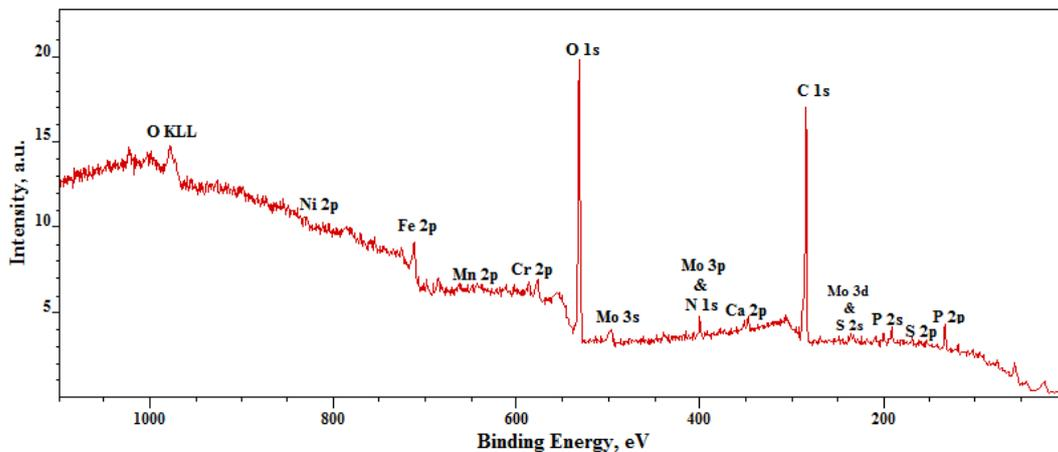
**Fig. 1.** XPS survey spectrum of both, passive carbon and contamination layers of AISI 316L surface electrochemically treated at 50 A/dm<sup>2</sup> in H<sub>3</sub>PO<sub>4</sub>, H<sub>2</sub>SO<sub>4</sub>, HNO<sub>3</sub> electrolyte mixture
