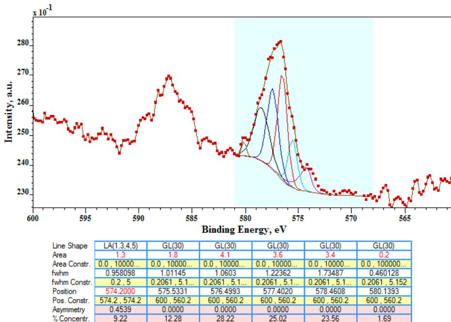
**Fig. 4.** Fitting of Cr 2p<sub>3/2</sub> spectrum of AISI 316L passive layer formed after electrochemical treatment
