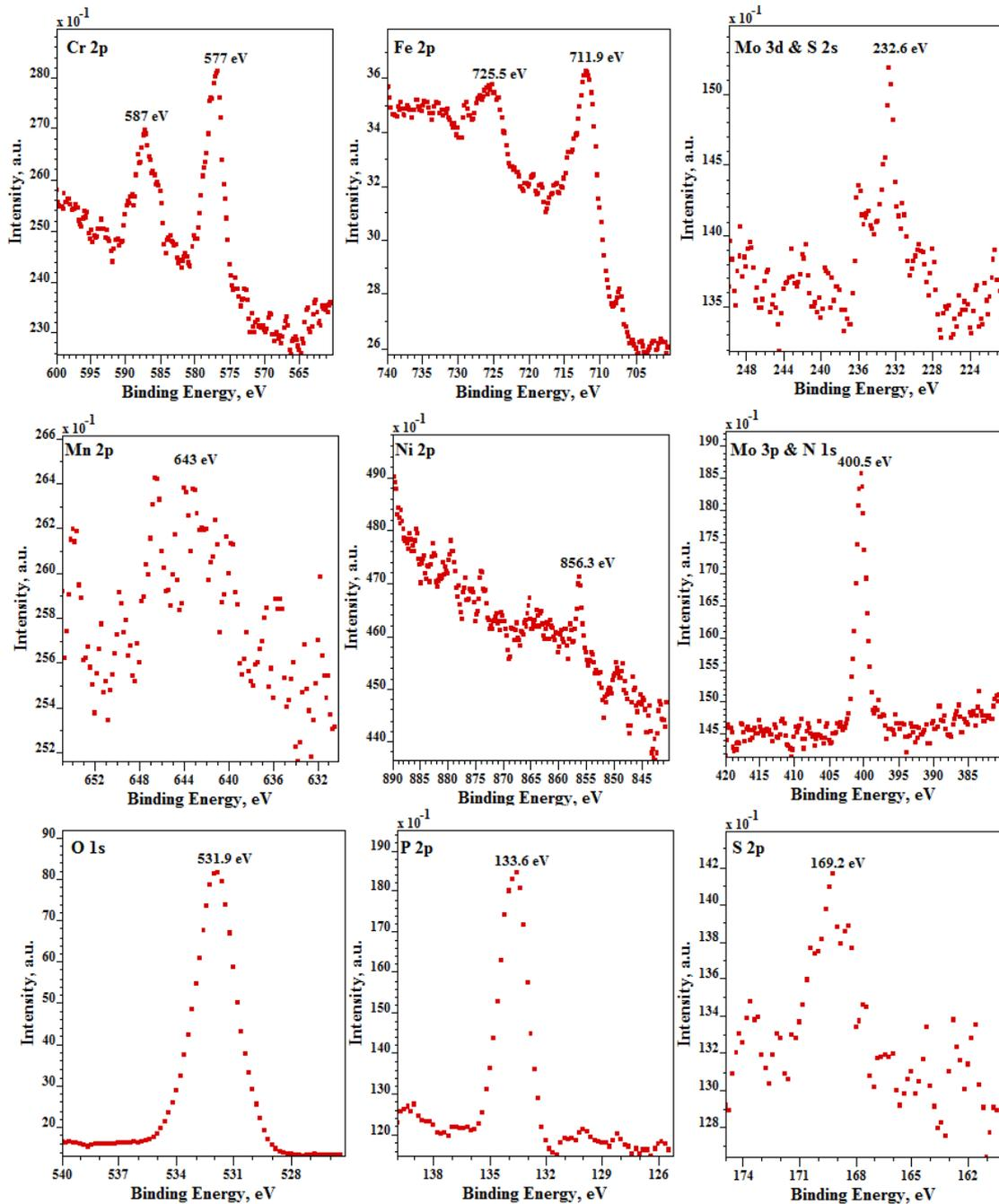
**Fig. 2.** High resolution XPS spectra of iron (Fe 2p), chromium (Cr 2p), molybdenum (Mo 3d), manganese (Mn 2p), nickel (Ni 2p), nitrogen (N 1s), oxygen (O1s), phosphorus (P 2p) and sulfur (S 2p) spectra of AISI 316L surface after electrochemical treatment at 50 A/dm<sup>2</sup> in H<sub>3</sub>PO<sub>4</sub>, H<sub>2</sub>SO<sub>4</sub>, HNO<sub>3</sub> electrolyte
