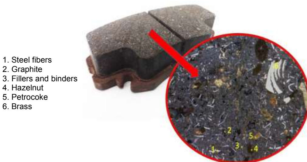
Fig. 5 The microstructure of brake pads produced with organic dusts
